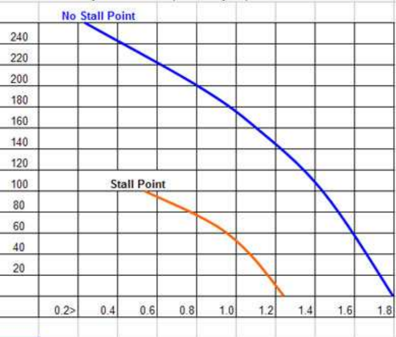
Both Fans - Input 250watts, 1360 r.p.m, 400mm Diameter
